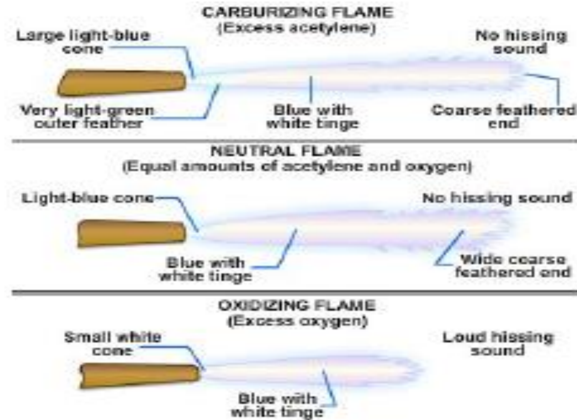
Fig: Example of carburizing, neutral, and oxidizing flames.
